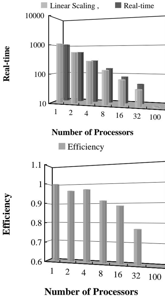
Figure 2: Timings (upper panel) and efficiency (lower panel) of parallel processing of the cloud model. The model used in the test had  $67 \times 67 \times 35$  grid points and was integrated for 50 steps on HITACH SR2201.
