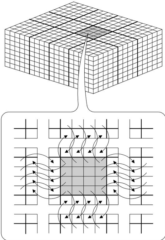
Figure 1: **Schematic representation of the domain decomposition and the communication strategy for the parallel computing.**
